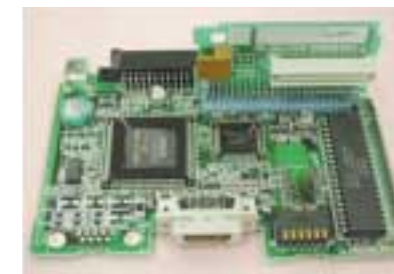
PLC using lead-free solder Model C200HE-CPU11
