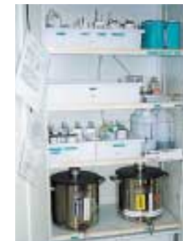
Chemical substances such as organic solvents are stored in a locked warehouse with partitions to prevent substance bottles from falling.
