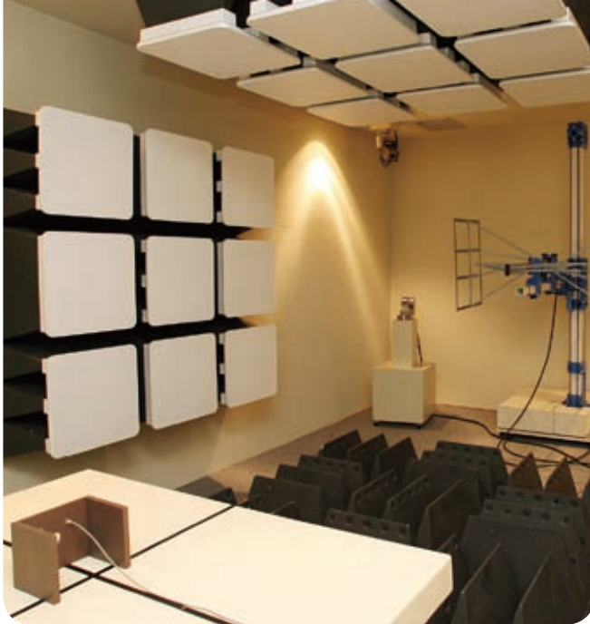
Measuring effects of electromagnetic interference from other devices on a product
