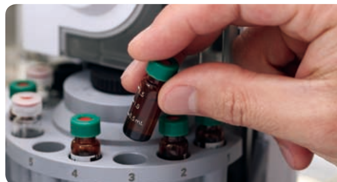
Ⓒ Inspection using an analyzer to ensure parts do not contain hazardous substances
