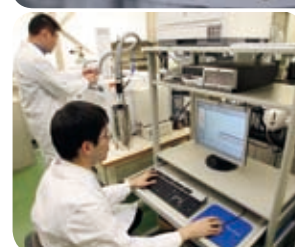
Ⓒ Inspection using an analyzer to ensure parts do not contain hazardous substances
